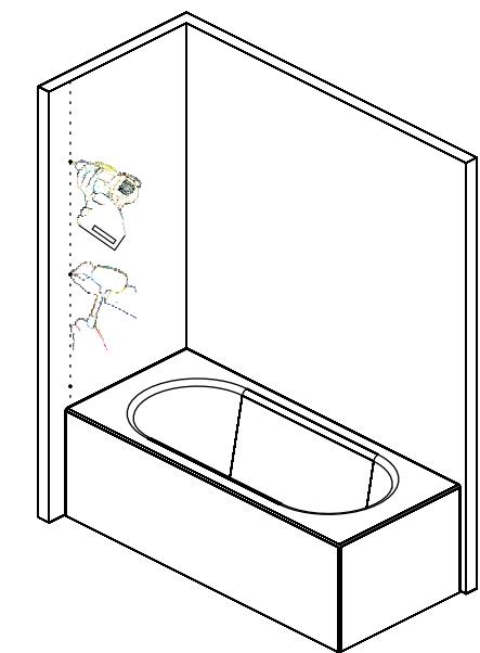
Drill holes and insert the wall plugs.
