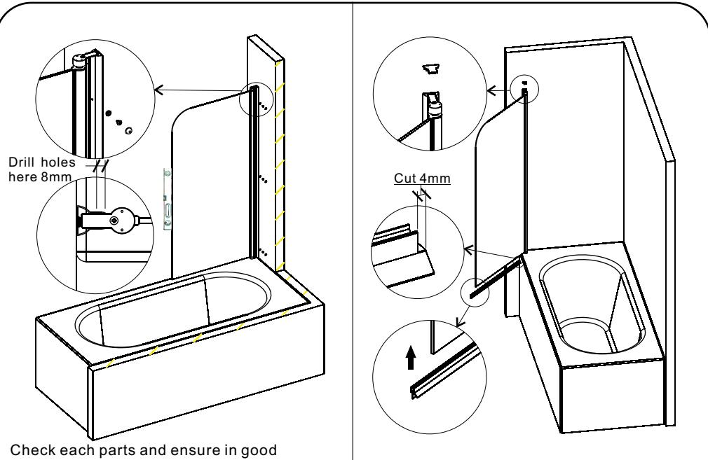
Check each parts and ensure in good parallelism and perpendicularity.
