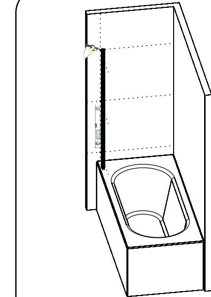
Mark out the holes on the wall.
