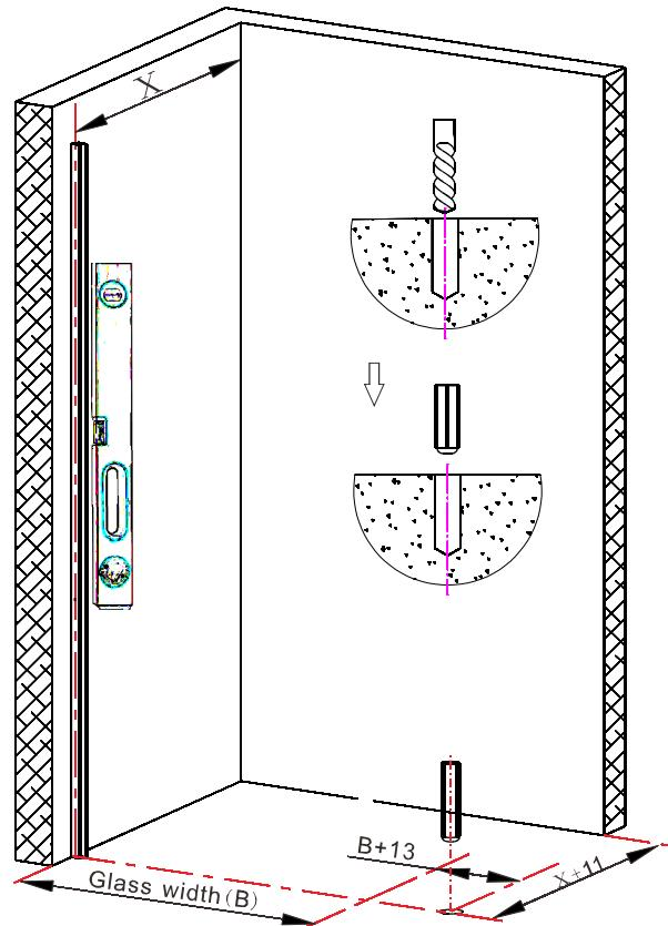
**Ensure the position of floor clip:** Confirm the hole of floor clip then drill hole for wall plug.
