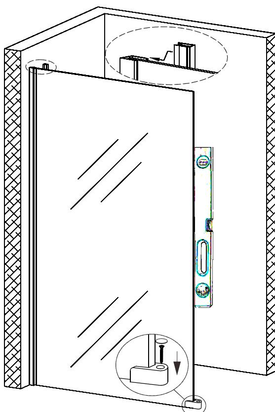
**Glass and floor clip installation:** Insert the glass gently to wall profile, then insert the press profile into wall profile. Please make sure glass is vertical. Finally screw the floor clip.
