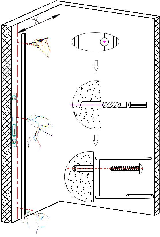
**Ensure the correct length of X:** Mark the hole on wall as per the hole in wall profile (Pay attention to the direction of wall profile). Then use  $\Phi 6$  drill bit to drill holes for wall plug. And fix the wall profile with round head screw . Attn. :  $X=1130\text{mm}$
