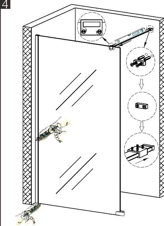
**Support bar installation:** Put the top clip of support bar on glass, ensuring the position of top clip and keep the bar leveled. Drill holes on wall for wall plug, then fix the pedestal on wall. Screw the wall connector and top clip tightly. Finally put silicon on glass bottom and do cleaning.
